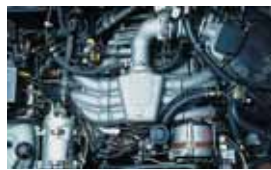
1986: Erster 6-Zyl.-Wasserboxer WBX 6 First watercooled 6-Cyl-Boxer WBX 6
