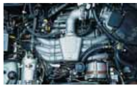
1986: Erster 6-Zyl.-Wasserboxer WBX 6 First watercooled 6-Cyl-Boxer WBX 6
